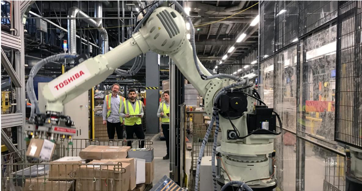
Robotic arm induction at the Montreal processing plant.
